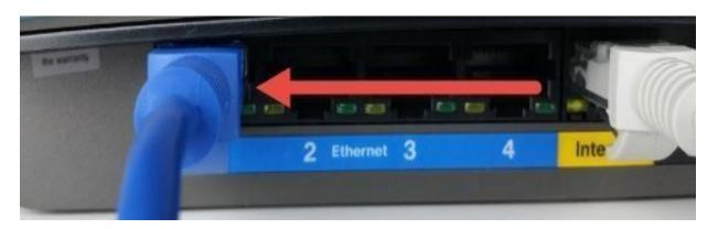
Then, connect the other end of the Ethernet cable to the DVR.
