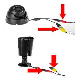
5. Secure the coaxial cable port from the camera to any of the video (coaxial) ports on the back of the DVR.
