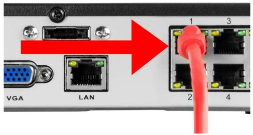
2. Connect the camera cable to an Ethernet cable.
