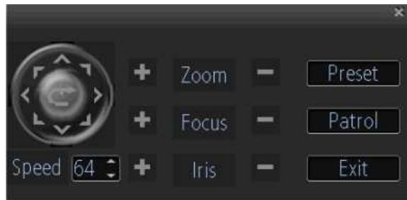
1. **Directional Pad/Auto-scan Buttons:** Controls the movement and direction of the PTZ. The center button is used to start PTZ auto-scanning.
