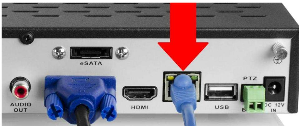
4. Connect the camera cable to an Ethernet cable.
