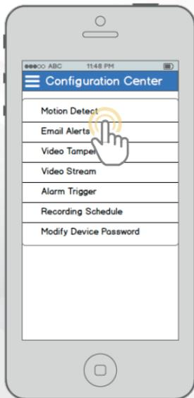
Tap "Motion Detect" to open the Motion Detection settings menu.
