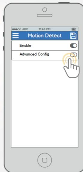
By default, motion detection is enabled. To configure advanced settings, tap the toggle switch in the "Advanced Config" row.
