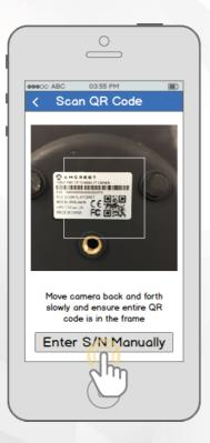
Scan the QR code (124) from the sticker on your camera. Move the camera or the phone to ensure that the entire QR code is visible and focused in the frame. In case the QR code cannot be scanned, please tap "Enter S/N Manually" to enter in the camera's serial number.
