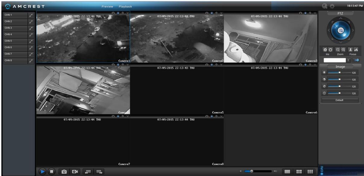
Preview: This tab shows live playback of any connected cameras. Ensure that the small icon on the left of each camera's name on the left hand list has a blue arrow icon present; otherwise the live video feed will not show.
