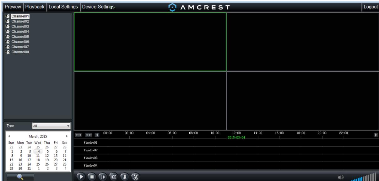
Playback: This tab allows for playback of recorded video. Select the date from the menu on the right and then click on the timeline at the bottom of the screen to select a playback starting location. Once the starting point has been selected, hit the play button to begin playback.
