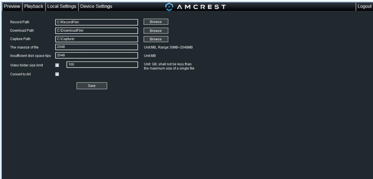
Local Settings: This tab allows for recording of the live feed to the computer that is accessing the DVR through the web.
